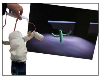
Figure 2. A tangible puppet equipped with sensors provides intuitive real-time control for the virtual Cactus Jack character in the Unreal game engine.
