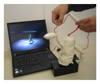
Figure 4. Users can pull directly on the marionette strings with a second hand to gain a greater range of independent arm movement beyond the paddle control.
